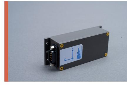
to commands to transmit data issued by an external computer. In the autosend mode, the Model 539 begins sending data as soon as power is applied to the unit.
