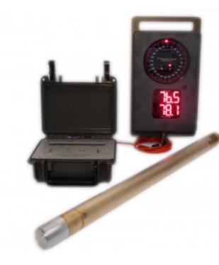
Downhole voltage, current draw and temperature are also displayed. The unit has a switch to zero the toolface angle at the surface before starting drilling or logging operations. During operation, toolface and inclination averaging can be used to dampen vibration noise due to drilling. This enables accurate orientation data to be obtained while continuing to drill.
