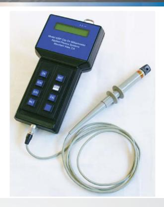
The Model 428P Portable Clip-on Milliammeter System is an accurate, sensitive ammeter designed to measure small currents without breaking or interrupting the current flow in a circuit. The current probe can be clipped onto wires up to 0.160" diameter; system accuracy is not affected by wire size.
